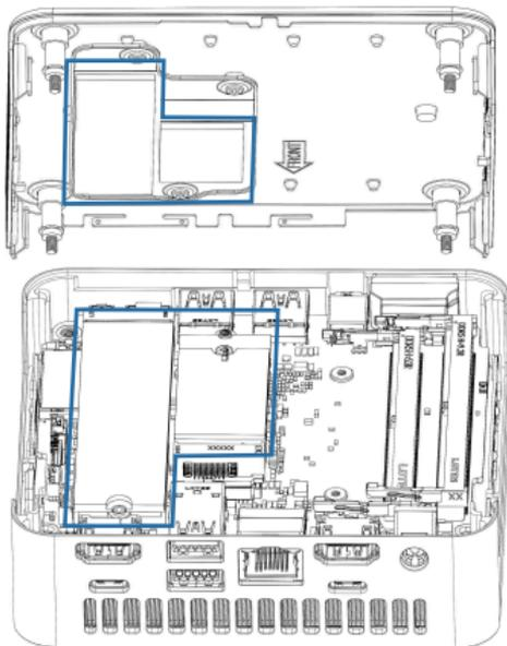
The SSD thermal grease on top of the case needs to be aligned with the SSD on the bottom.
